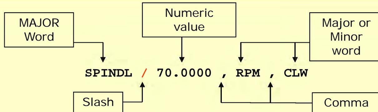
In ISO, this APT command turns on the spindle clockwise at 70.0000 RPM. On most ISO controllers, a post-processor would translate this as:
